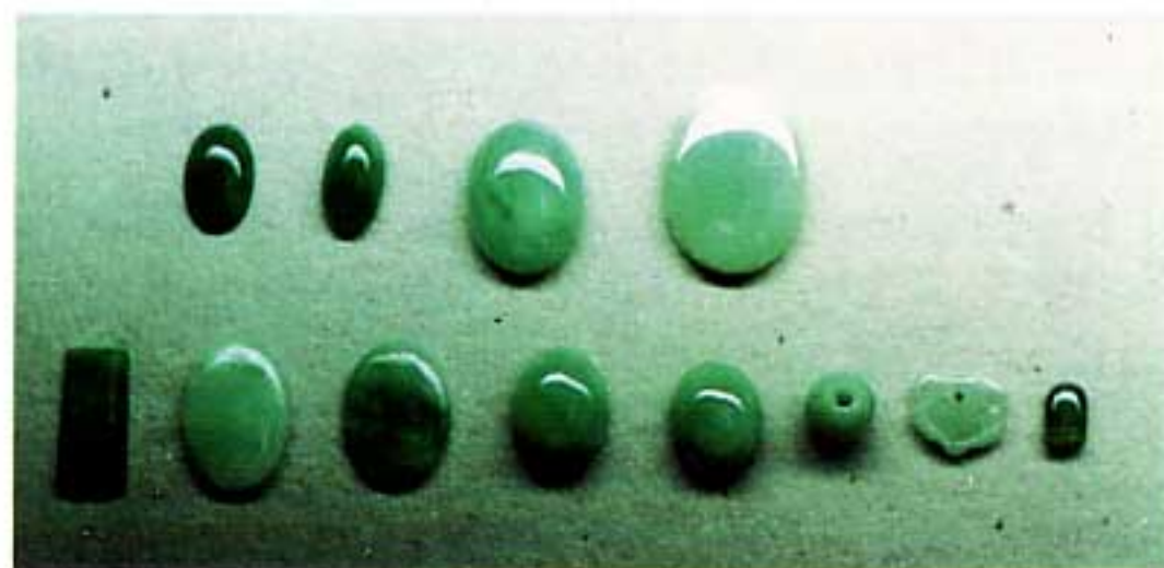
Fig. 1. Eight pieces of bleached polymer-impregnated jadeite (lower row), and four pieces of natural jadeite (upper row). For identification purposes the jadeites have been numbered left to right 1-4 (upper row), 5-12 (lower row).
